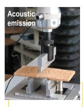
Combining acoustic emission with mechanical tests can be applied to predict the textural attributes of foods
