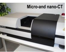
Micro- and nano-CT allow scanning real samples in 3D under normal environmental conditions without any preparation techniques
